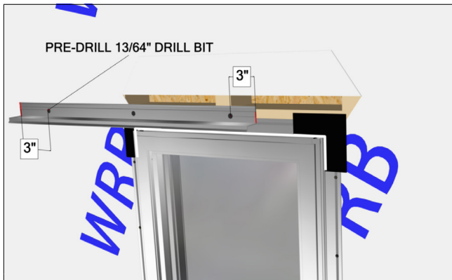
Fig 11. Once sealant is applied everywhere that will contact the nailfin, predrill the drip cap using a 13/64" drill bit. The holes must be 3 inches from each edge of all nailfins, followed by 12 inches on center for each next hole.
