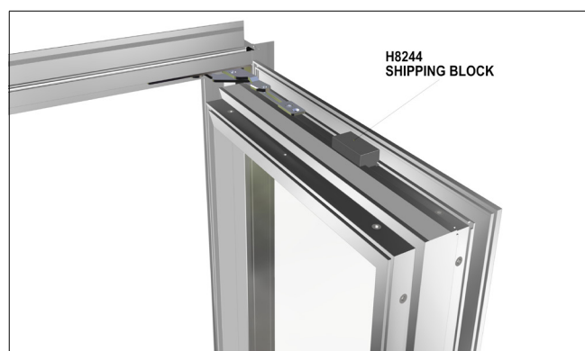
Fig 17. Remove the Shipping Blocks located on top of the sash. Slide it out, and dispose.
