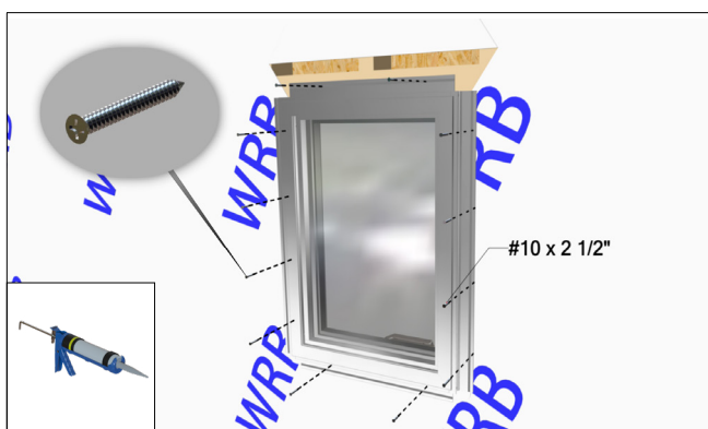
Fig 7. Fasten the frame to the rough opening through the predrilled holes on the nailfins, using the recommended #10 x 2 1/2" screws. If the unit gets a drip cap, do not fasten the nailfin at the head in yet.
