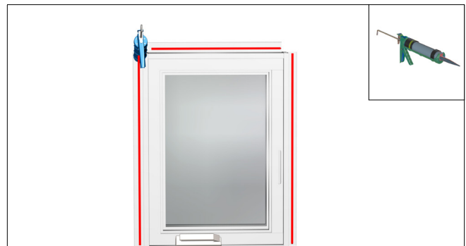
Fig 4. After pre-drilling, apply sealant along the interior of all 4 nailfins.
