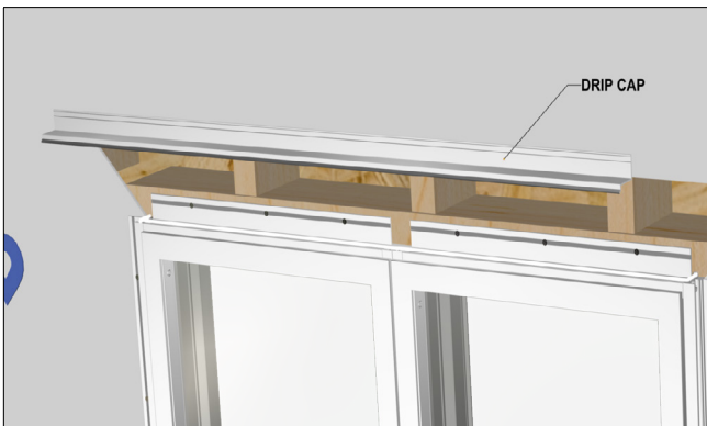
Fig 7. After applying sealant, place the drip cap on top of the frame, and make sure it's flush with the nailfin and the frame.
