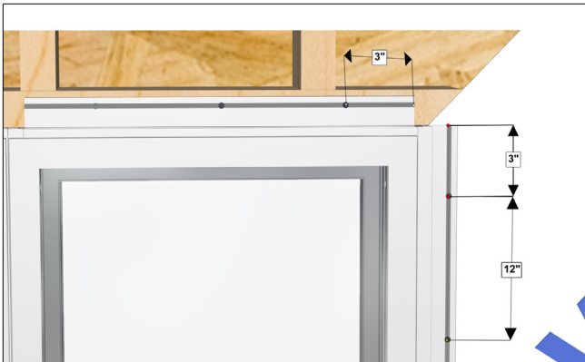
Fig 5. The first screw should be 3" from the corner, followed by 12" off center for the next screw.
